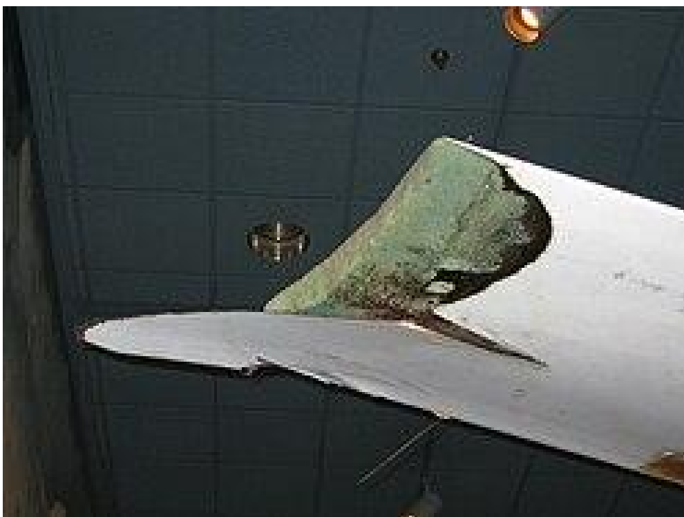
Damaged left wingtip
