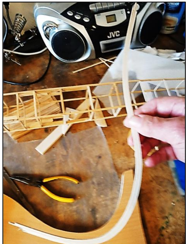
Making a laminated shape for the new underbelly.
