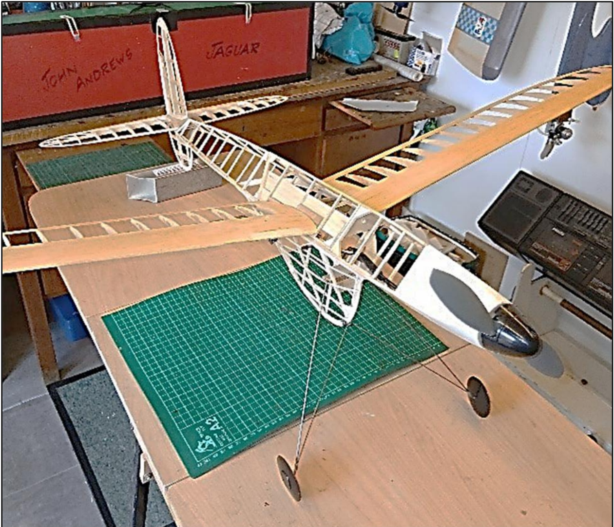
Most of the reinforcement repairs done, motor and speed controller fitted next job is to install servos and control rods.
