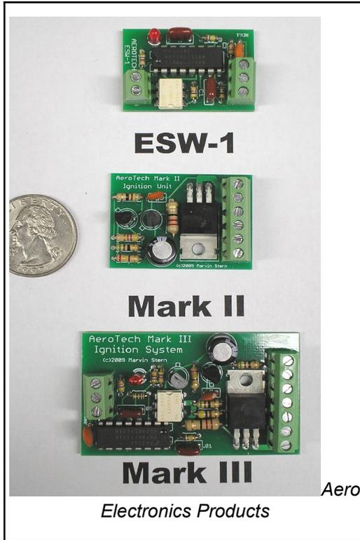
Replacing it are two new products. The first is the all new Mark II Ignition Unit. This is a standalone unit and does not include the ESW-1. The major feature is the protection afforded the output transistor and ignition coil in the event the engine stops prematurely with the points closed. If this happens, the unit shuts down immediately protecting the unit from possible overload and the ignition coil from burning up. It measures approx. 1-1/8 x 1-1/2 inches.
