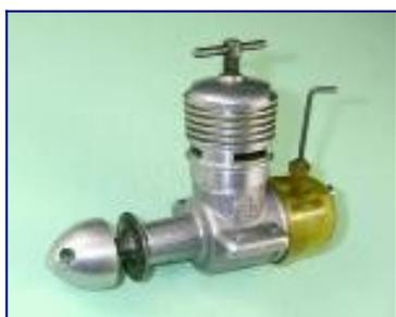
As an RRV engine, the Hornet was a design derivative of the Bee, but utilized the simpler radial porting arrangement of the Baby. No provision had been made in the displacement-oriented "Mark" number sequence for these new models, so rather than revising the system E.D. simply allowed the Mark number scheme to die, quietly removing references to
