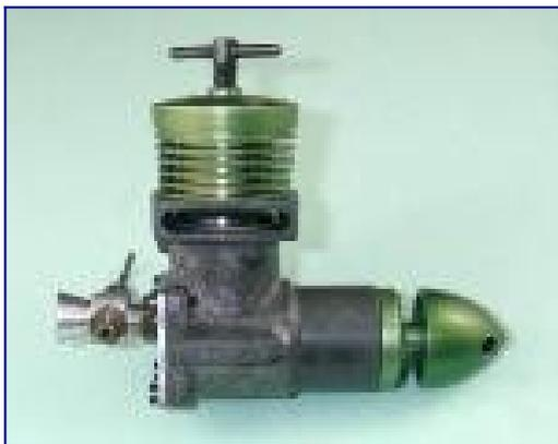
The Fury looked like a scaled-down version of the Racer but was equipped with reed valve induction. An unadvertised but very similar 2.46 cc green-headed reed valve version of the Racer had been produced in very small numbers beginning in 1957, and this was to remain available to special order until 1961.
