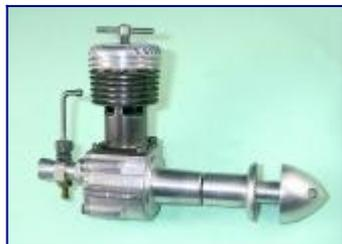
October 1949 saw the introduction of the E.D. Mk IV "Three-forty-six", a rear rotary valve (RRV) 3.46cc diesel with a single ball-race crankshaft later named the Hunter. Due to teething problems with the production of the die-cast cases for this model, the initial production batch used barstock cases.
