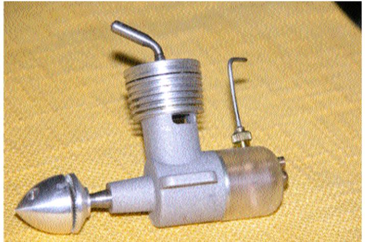
Drone fixed head diesel, scaled to point five
