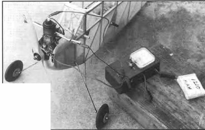
*Bob's clip-on ignition system for troubleshooting on-board components and wiring. Switch off the internal system first. If the motor runs properly with the clip-on attached, it's a pretty good sign there's something wrong with the internal system. In the text, Bob explains how to diagnose the situation using this device.*
