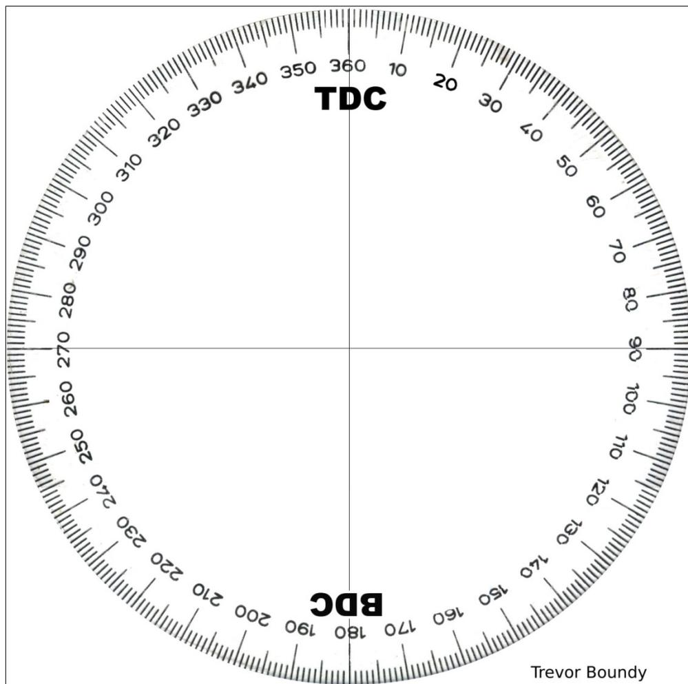
The wheel can, of course, also be used for checking engine port timing and dwell if you’re into more extensive engine work.
