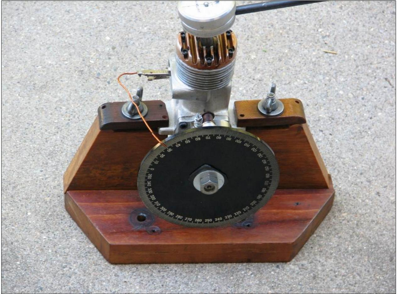
This view shows the indicator wire in place, along with the dial gauge for establishing TDC. The dial gauge isn't locked in, but is just hand held solidly in place while rotating the wheel and taking readings.
