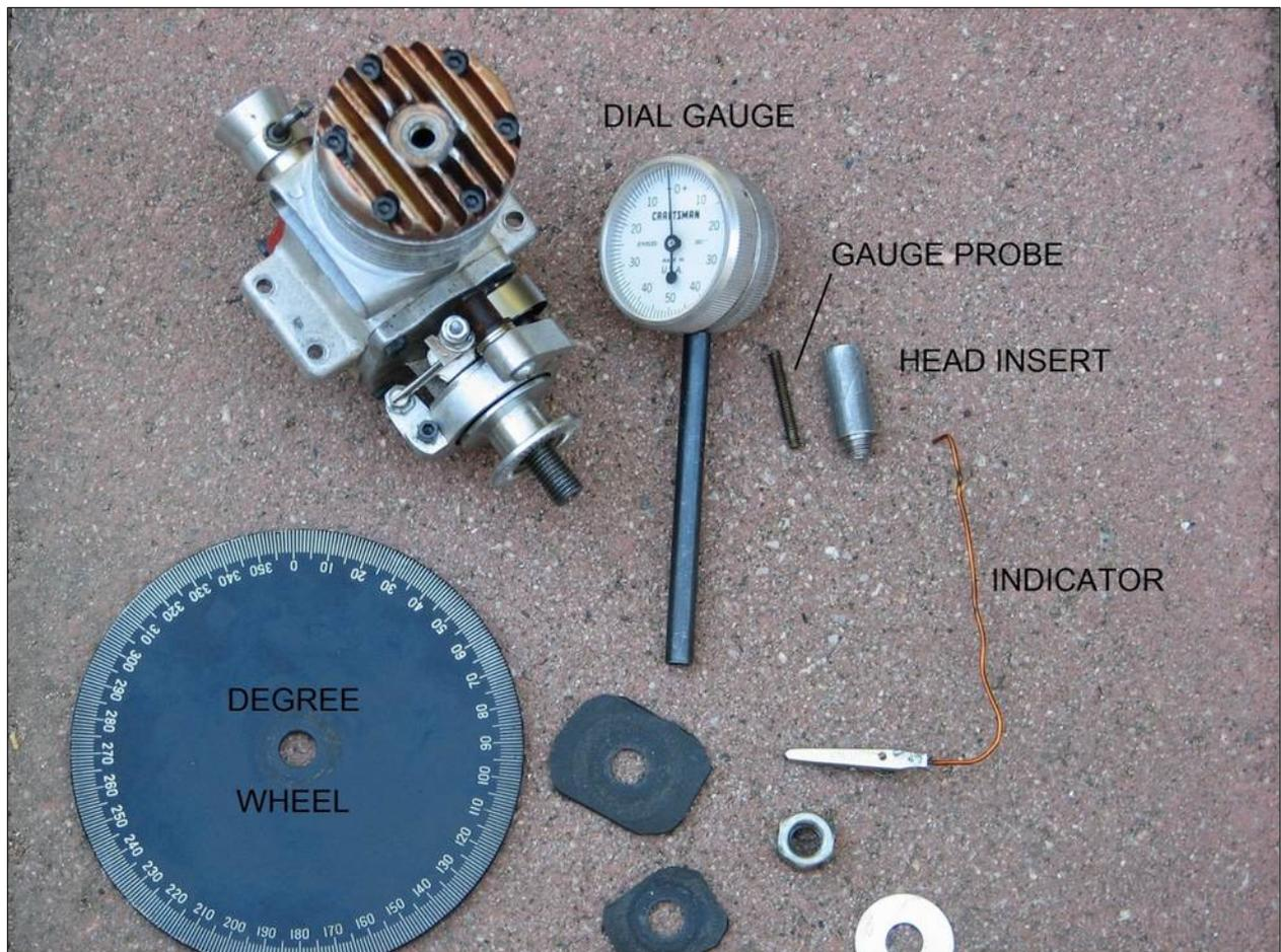
Well, actually it shows a bit more than what's really needed. The machinists dial gauge gives a more accurate reading of the piston's top dead center (TDC) location, but isn't strictly necessary. The gauge probe and head insert had to be custom made to use the dial gauge. The head insert screws into the spark plug hole. It's hollow to allow the longer than stock gauge probe to reach in and touch the piston top. I made an insert for each of the two plug sizes.
