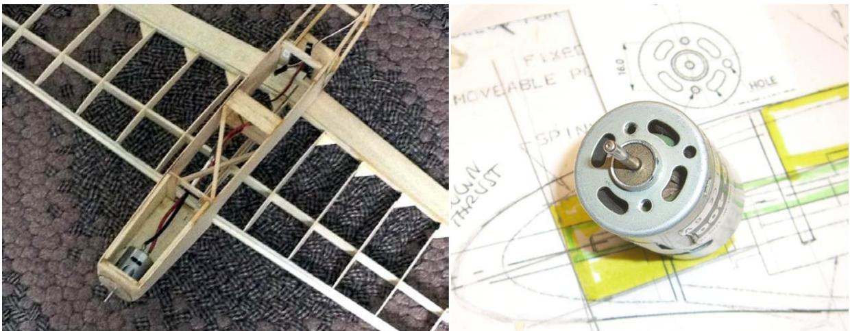
If you are converting a 1/2 A Cox powered airplane you can buy mounts that will attach your Speed 400 to the Cox bulkhead. The prettiest of these mounts is made by Loren Kramer especially for this purpose. Here is one of his mounts used by Tandy Walker on one of his models. You can reach Loren at;
