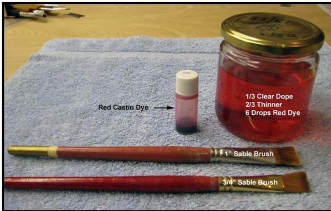
One coat of the red tinted clear dope mixture was brushed onto the silk. The results are shown in the picture below. The silk is actually a deeper red that the picture shows probably due to the florescent lighting in the model room. Here is where the undercoat of Polyspan Lite really pays off. One coat of red tinted clear dope mixture basically filled the grain of the silk with no unsightly globs or drip throughs on the underside of the silk.
