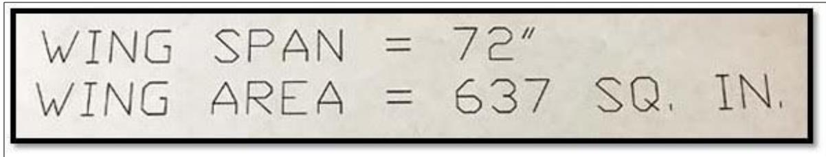
The wing's half-span of the printed plan was carefully measured to be 35.81" (71.62" full span). I sent this measurement and the wing plan PDF file to my friend Alfredo Herbon in Argentina to calculate the wing area using his ACAD program. Alfredo's results shown below calculated the area to be 635.98 sq. in. The model's **Aspect Ratio** =  $(\text{Span} \times \text{Span}) / \text{Area} = (71.62 \times 71.62) / 635.98 = 8.065$ .
