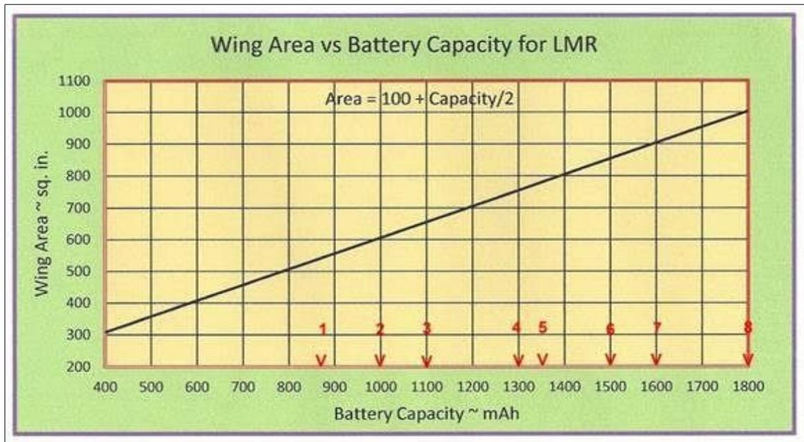
This sizing chart was used to determine wing area estimates for each of the 8 battery packs, which are presented follows:
