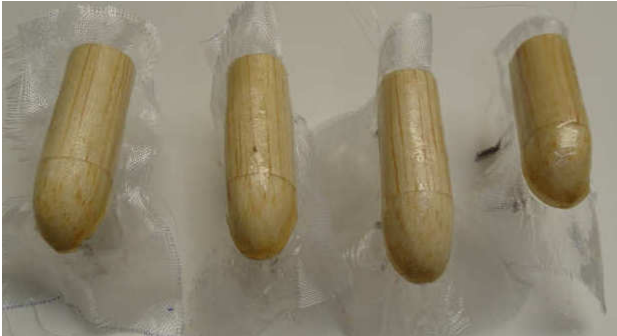
Figure 7 The housings are now covered with very light fiberglass and 30 min. epoxy. Excess epoxy is squeegeed off. I have set the housings up on T pins stuck in my work board while the epoxy sets.
