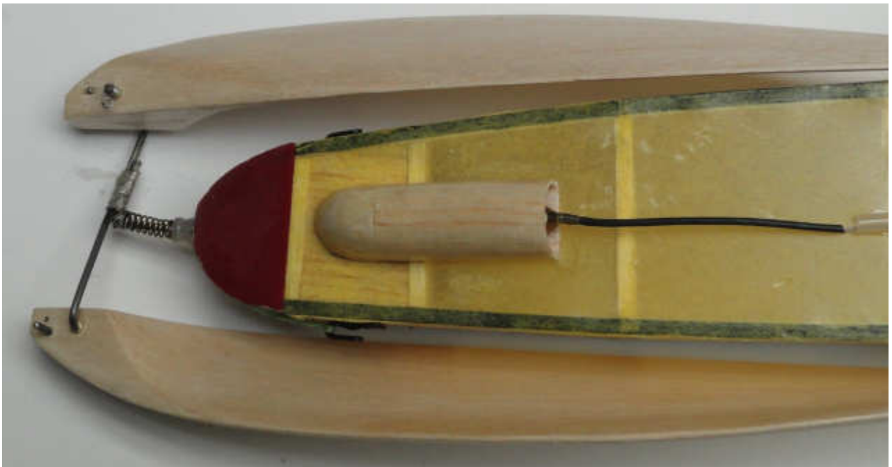
Figure 8 Here is a completed housing in stalled on my Moffett. The excess fiberglass has been trimmed and the housing lightly sanded.
