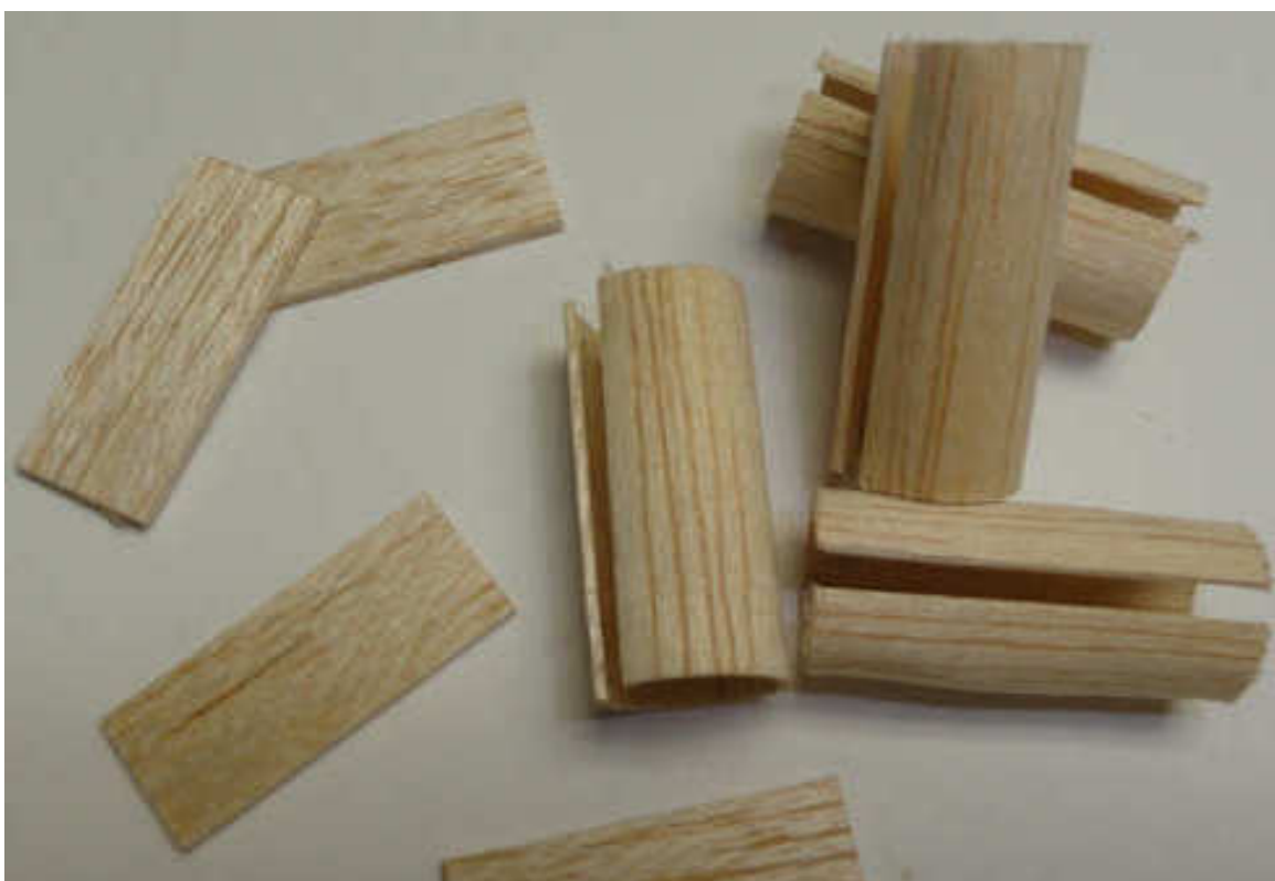
Figure 4 The 1/32 balsa tube is cut to length. The rectangles are 1/16 and will serve as the base of the housing.
