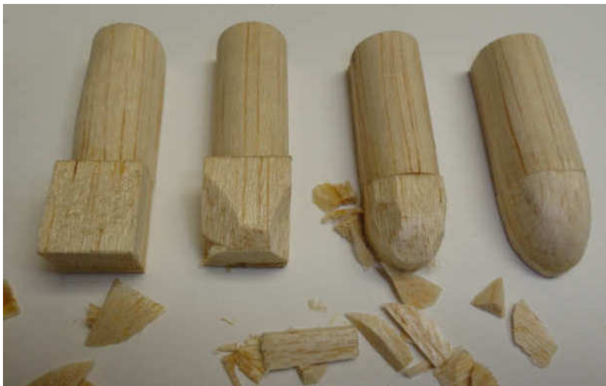
Figure 6 Glue a block on to one end of the housing. Carve to shape, sand, dope, sand, dope again and sand lightly.
