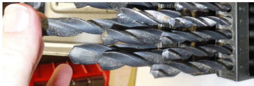
Figure 2 I select a drill about the same diameter as the tx is wide.
