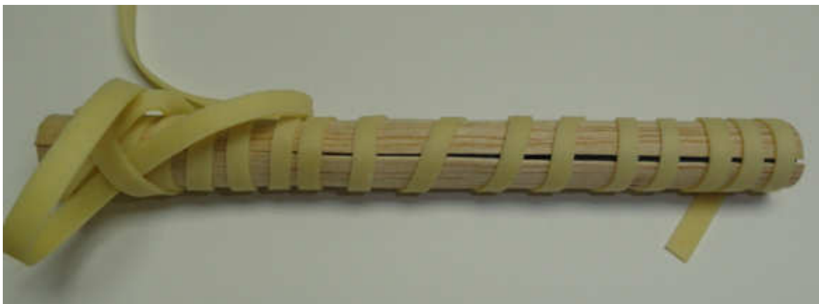
Figure 3 After soaking 1/32 balsa in hot water, it is wrapped around the drill, secured with scrap rubber, and left to dry.
