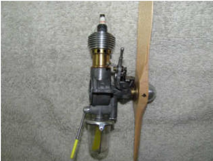
This Bill Schmidt's latest project, a first model Atom – 0.9 displacement ignition engine – ask how he makes it so pretty! Notice that plating!
