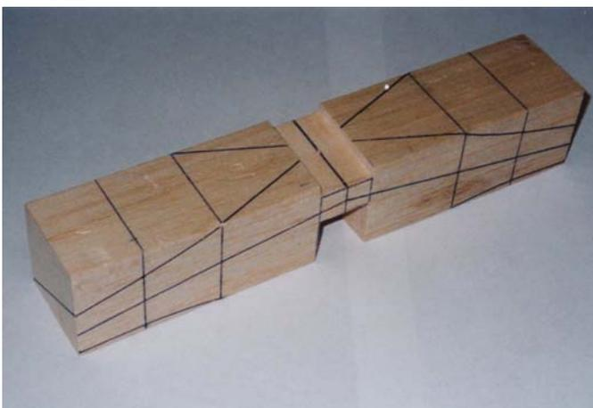
The block marked out with hub cut back
