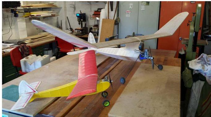
A new duration model was called for – so after much scrotum scratching I decided to build a new fuselage for my old %85 bomber after its oil soaked pylon fell off. The reasoning being I already had a solid wing and I could build a new fuse with removable tail for transport. Good old doculam was used to cover my dodgy woodwork and a couple of Savox mini's fitted in the Stab. I dusted off a barely run-in ASP61 FS and nailed it to the front. Ready for testing!
