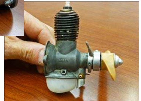
Left: Another of Lescher's beauties. This one a Torpedo .23 RC with radial mounting adapter
