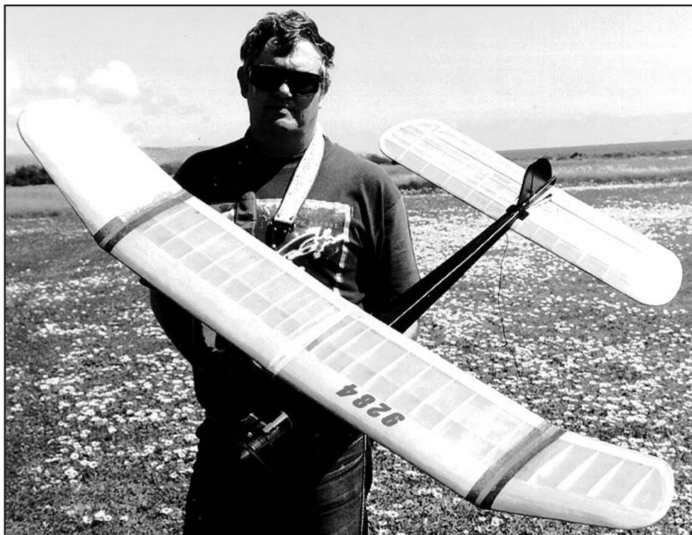
inches and all up weighed only 12 ounces, being powered with a quite potent Elfin 2.49 (radial mount). This engine was also used in the "Super Thermic" of Max Nicol that won open power at the 1952/3 Bendigo Nats. The original "Jaded Maid" was quite fragile, needing to be reinforced in the wing and pylon for the R/C Burford event. DH.
