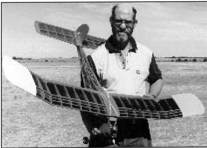
Kevin Fryer , President SAM 600 with his enlarged "Atomizer" for the Burford Event. Taipan 2.5cc plain bearing diesel, 9x4 Master airscrew. Model flew well.
