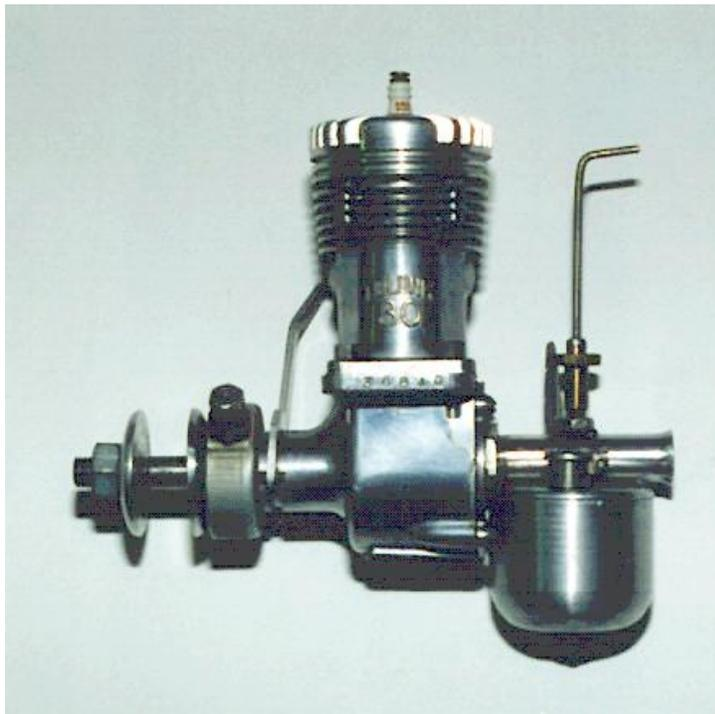
And here's a Delong 30, which features rear disc rotary induction, similar to Hornet, McCoy, Dooling, etc. Although it's not quite in the same performance class, it's still a good strong running, nice handling engine.
