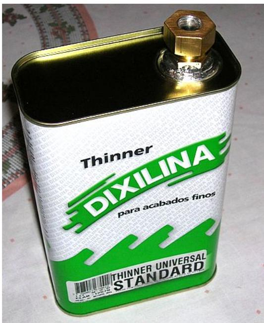
Here is Alfredo Herbon's solution to keeping ether contained. He solders brass fittings made for household natural gas lines onto a clean can.
