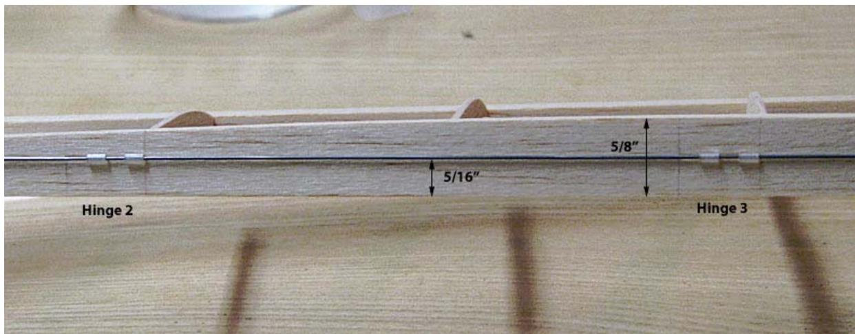
**KLETT HINGES:** Here's how Tandy Walker installs those two piece hinges. It's also the way I and probably others have always done, so naturally I think it's a bright idea. By inserting the long piece of music wire before gluing them in place, you are assured of a straight no bind alignment. When you install the other halves, you still use the wire and slide everything into place before gluing them in.
