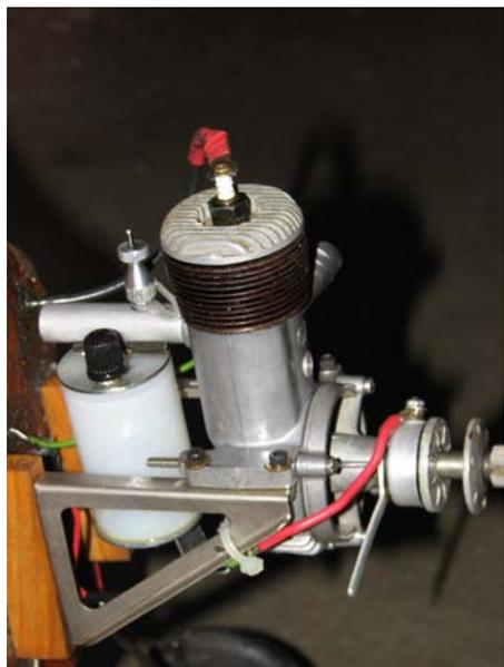
This illustrates both the tips above. The plastic zip tie at the aft end of the red point wire reduces the wires vibration but still lets the timer move for adjustment.
