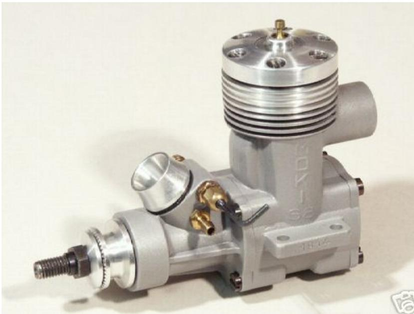
This Moki Schnuerle has three bypasses. The larger one is in the same place on the left side as the engine above. There are also two extra bypasses called boost ports fore and aft. The forward one is visible in the picture. The main bypass on a Schnuerle doesn't shift if the exhaust direction shifts. That's because the main bypass entry would be partly masked by the crank web. The boost port intakes sit higher in the sleeve and are above the crank web.
