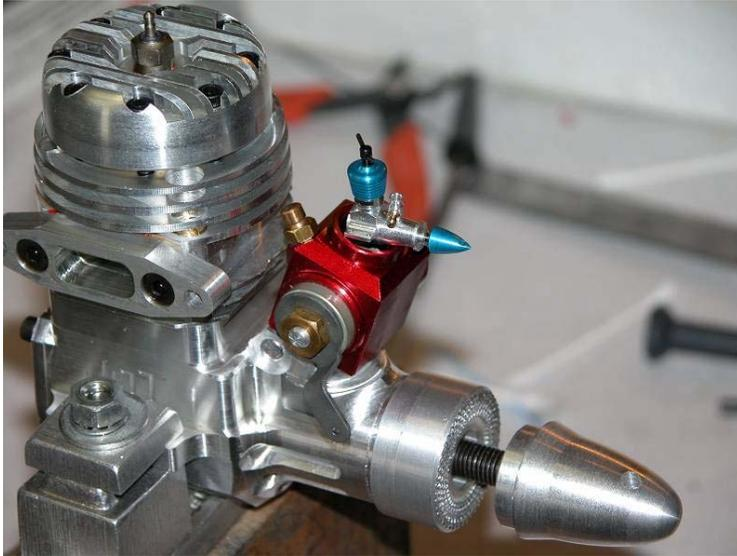
**SMALL DIESEL!** Wait, take a closer look. That's a 60 size glow engine with the small diesel almost swallowed up in the carburetor.
