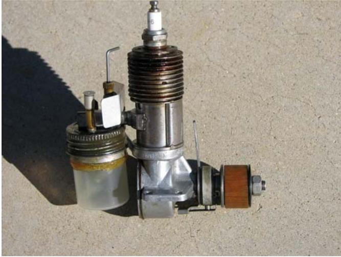
Here's that Brown junior exhaust deflector mentioned earlier. It doesn't restrict exhaust flow nor cause hot running as did those restrictive little clamp-on exhaust pipes. It's held on by the spraybar and has extended "legs" down around the intake tube to prevent rotation.
