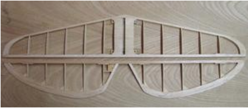
Stripped, Re-glued, and refinished Horizontal Tail
