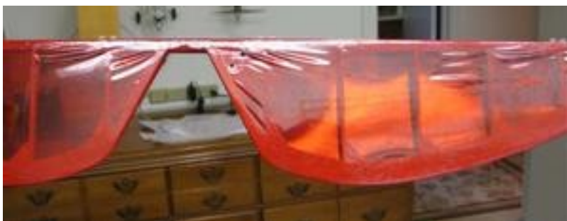
Recovered Stressed Elevator and Stab
