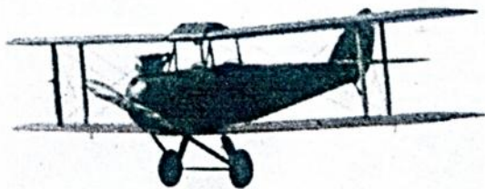
One of the first batch of Moths with an unbalanced rudder. Photograph by courtesy of the Director of the Science Museum.
