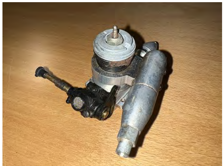
The "what is it" turned into a show and tell item is a Cox .074 Queen Bee, production started in 1987.
